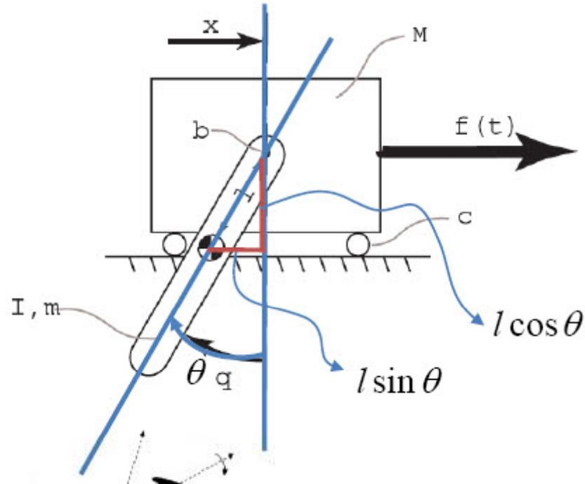
$$\begin{aligned} (M + m)\ddot{x} + c\dot{x} - ml\ddot{\theta} &= f(t) \\ (ml^2 + I)\ddot{\theta} - ml\ddot{x} + mgl\theta + f_{\theta}\dot{\theta} &= 0 \end{aligned}$$
